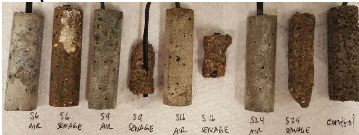
Figure 2. Appearance of harvested concrete coupons subjected to soaking in ultra-pure water for analysis of products excreted by biofilm present on the coupon surfaces (BIT Table 2 and BAT Table 1 data) . Sample from S16 sewage was split at a crack to create two samples for analysis. Sample S6 shows the presence of fats, oils and grease (FOG) on the surface of the coupon. Photo was taken three days after analysis and does not necessarily represent condition of the coupons immediately after analysis.
