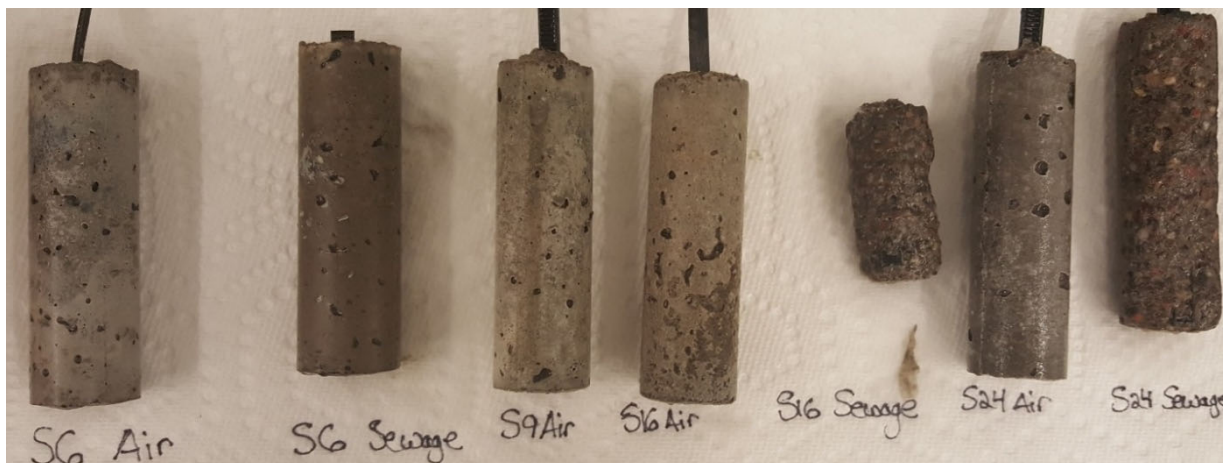
Figure 1. Appearance of harvested concrete coupons subjected to direct lyse (BIT Table 1 data). No sample was available from S9 sewage for analysis. Sample from S16 sewage was split at a crack to create two samples for analysis.
