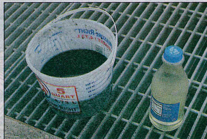
This photo shows “before” and “after” water is treated by the Crane Engineering Mobile Septage Treatment System, a new sanitation technology that processes human fecal sludge into non-potable water for agricultural or industrial use.
