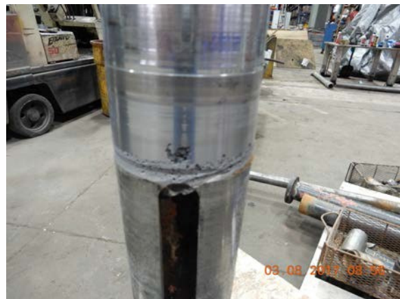
Pump Shaft: Has deep grooves in bearing journals from wear. Shaft also has pitting from corrosion.
