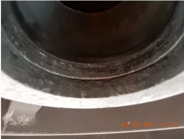
Diffuser Bowl: The restrictor bushing and snap ring groove fits are washed out.
