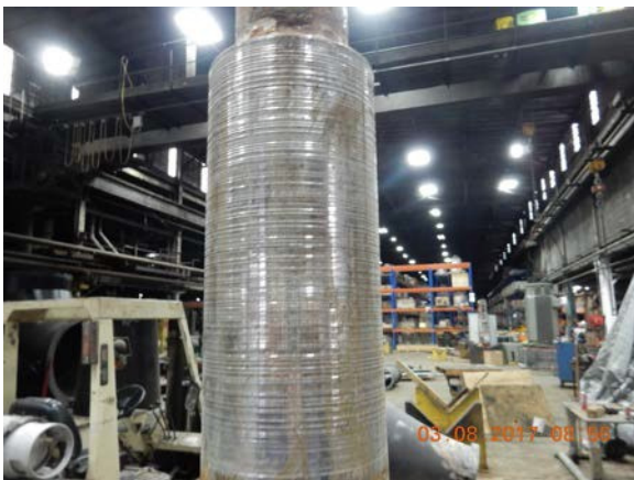
Pump Shaft: Has deep grooves in bearing journals from wear. Shaft also has pitting from corrosion.
