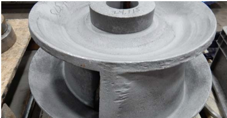
Impeller: Hub requires repair and will be ceramic coated per the original quote.
